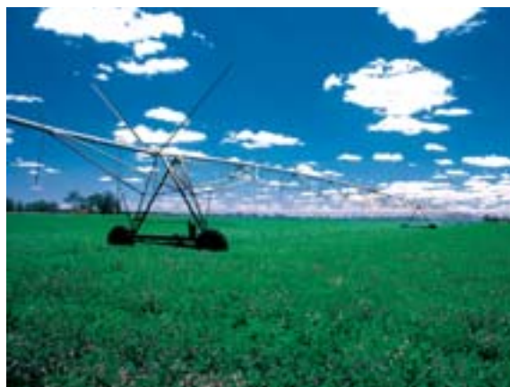
Figure 18. Sprinkler irrigation is more efficient than flood irrigation, but less efficient than drip irrigation.
