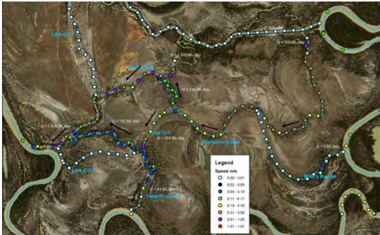
Figure 7-9: Hydrodynamic modelling of CCB Creeks system showing mean velocity within the channel with inflows of 1,500 ML/d at Carrs No. 1 and 500 ML/d at Carrs No. 2 [NSW Public Works - FCS 2013]
