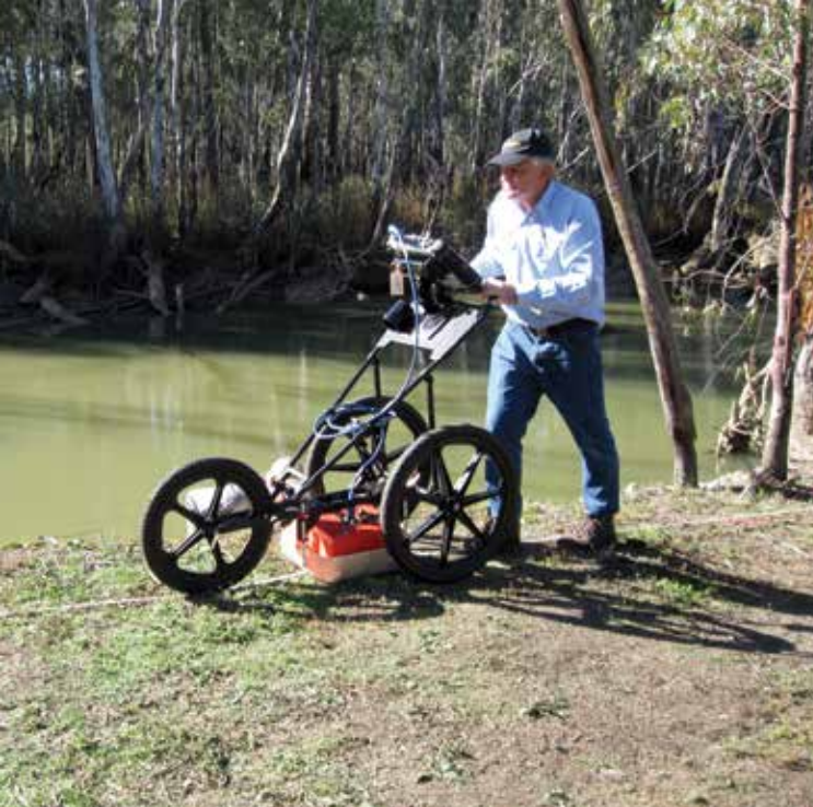
Use of Ground Penetrating Radar (GPR) (NPWS 2018)
