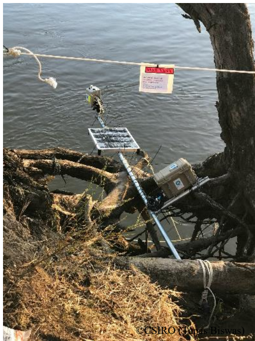
Figure B1. The installations of HydraSpectra at Tocumwal Site 1 (left, HS15) and Barmah Site 3 (right, HS16). HS15 and HS16 are serial number for the equipment.
