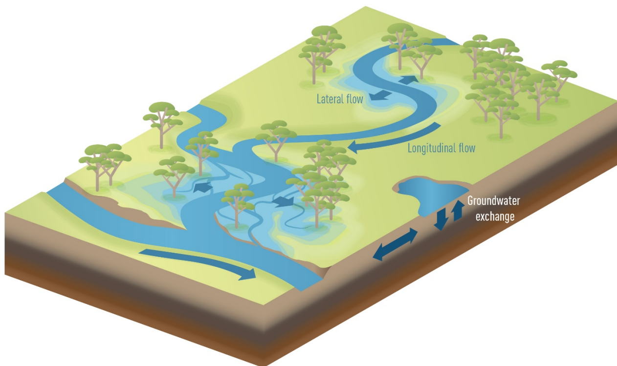
Figure 12: Conceptual diagram of the longitudinal and lateral connectivity of flows in a river system
