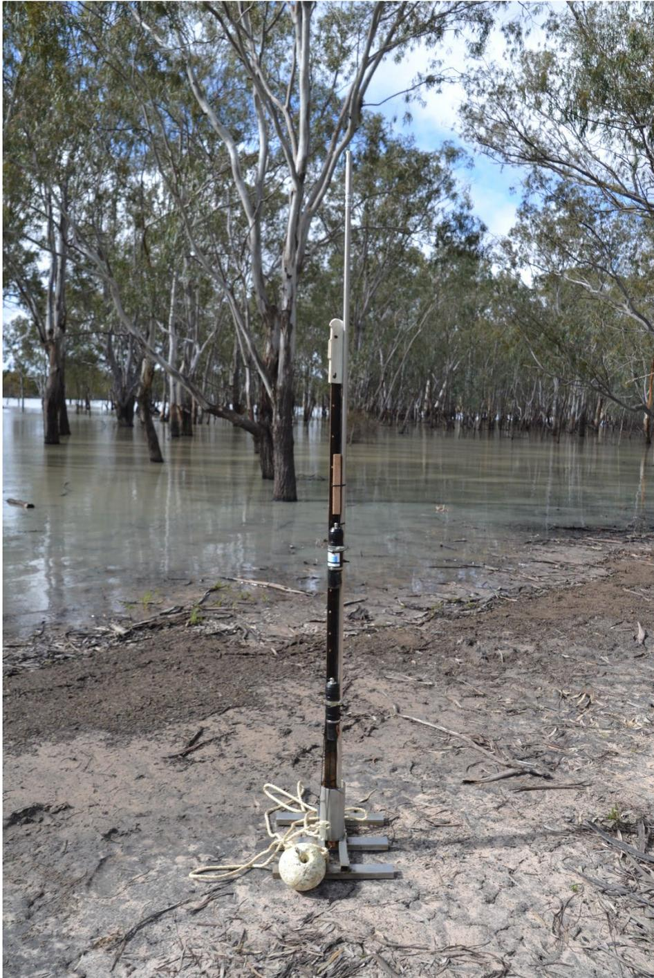
**Figure 1. Photo of logger station with two D-OPTO loggers (0.4 m and 0.8 m above base) and Trutrack water level logger, prior to deployment.**
