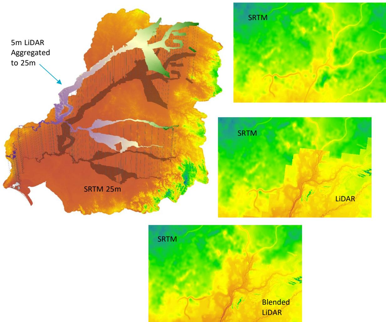
**Figure 1 Merging LiDAR DEM and SRTM: the original SRTM and LiDAR DEM are shown in the large map on the left; the top right insert shows a zoomed in view of SRTM; the middle insert shows the abrupt change (local steps) at the boundary of the two datasets; the bottom insert shows the merged data with the abrupt change removed.**
