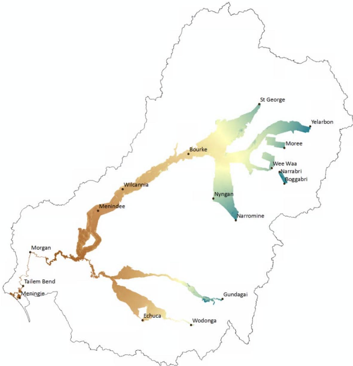
Figure 2 Merged LiDAR DEM with a gap in the Namoi between Narrabri and Wee Waa.
