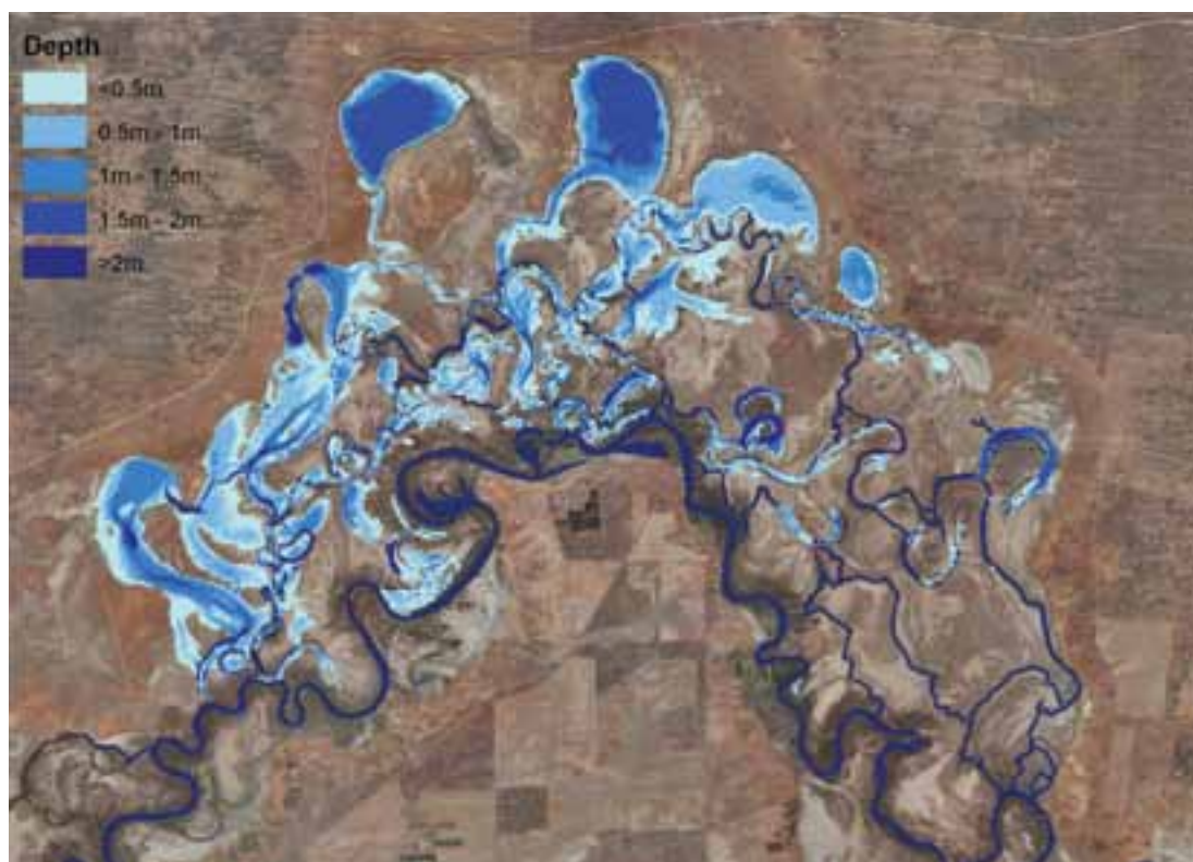
Figure 4.3: Inundation with the regulator in operation at 10 GL/d and raised to 19.87 m AHD
