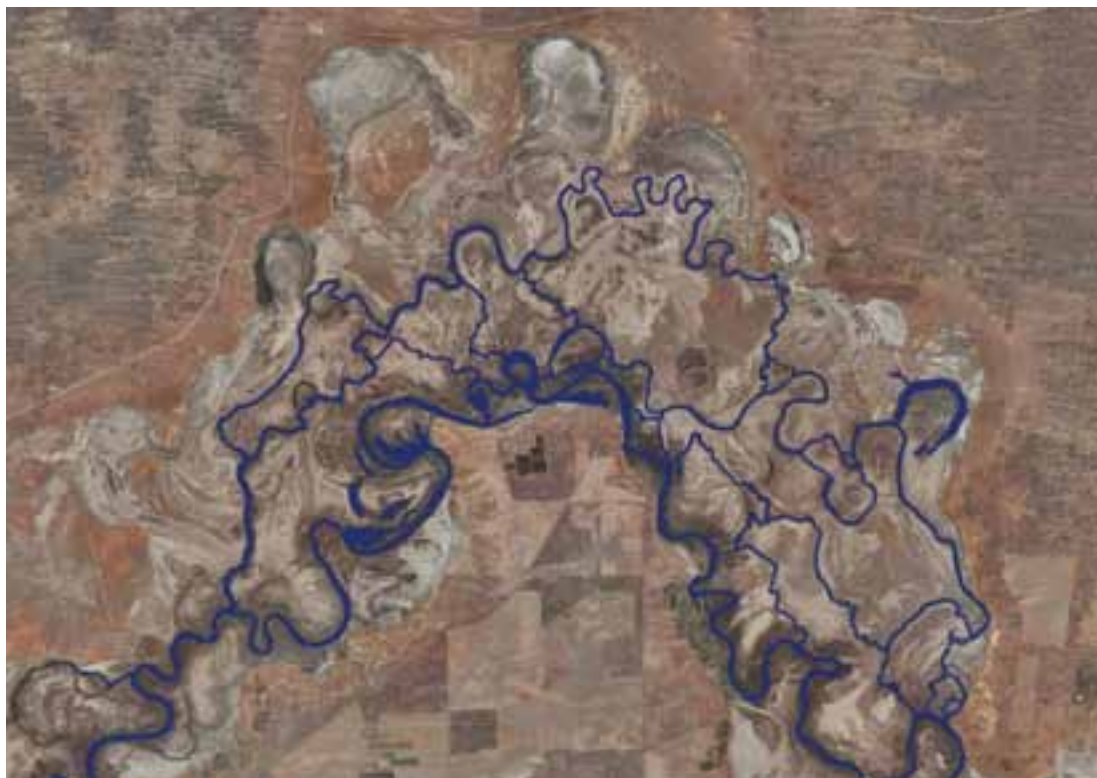
Figure 4.2: Inundation at 10 GL/d without the Chowilla regulator
