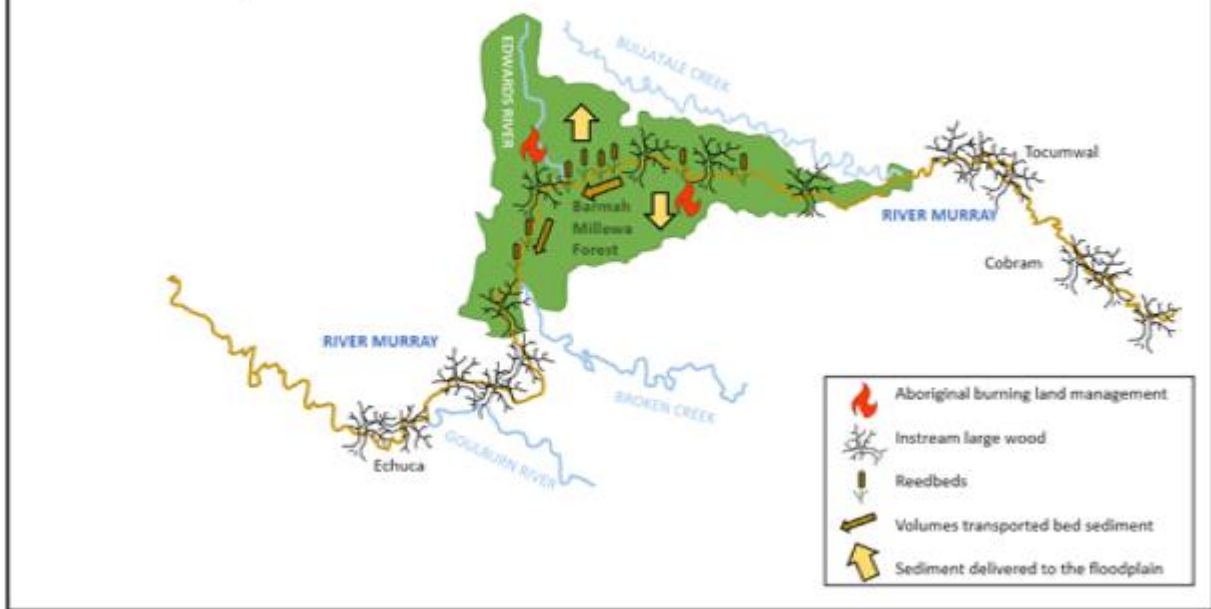
Figure 24. The pre-European reference condition of the River Murray and Barmah-Millewa Forest. The River Murray is brown to signify that it conveyed sediment, and the width of the line and arrows indicate relative volumes of sediment, the lighter colour being mainly suspended sediment. Snags were present in the channel, rushes were more extensive, sediment volumes into the reach were low and proportionally higher in suspended sediment with high losses onto the floodplain, land management was Aboriginal burning.
