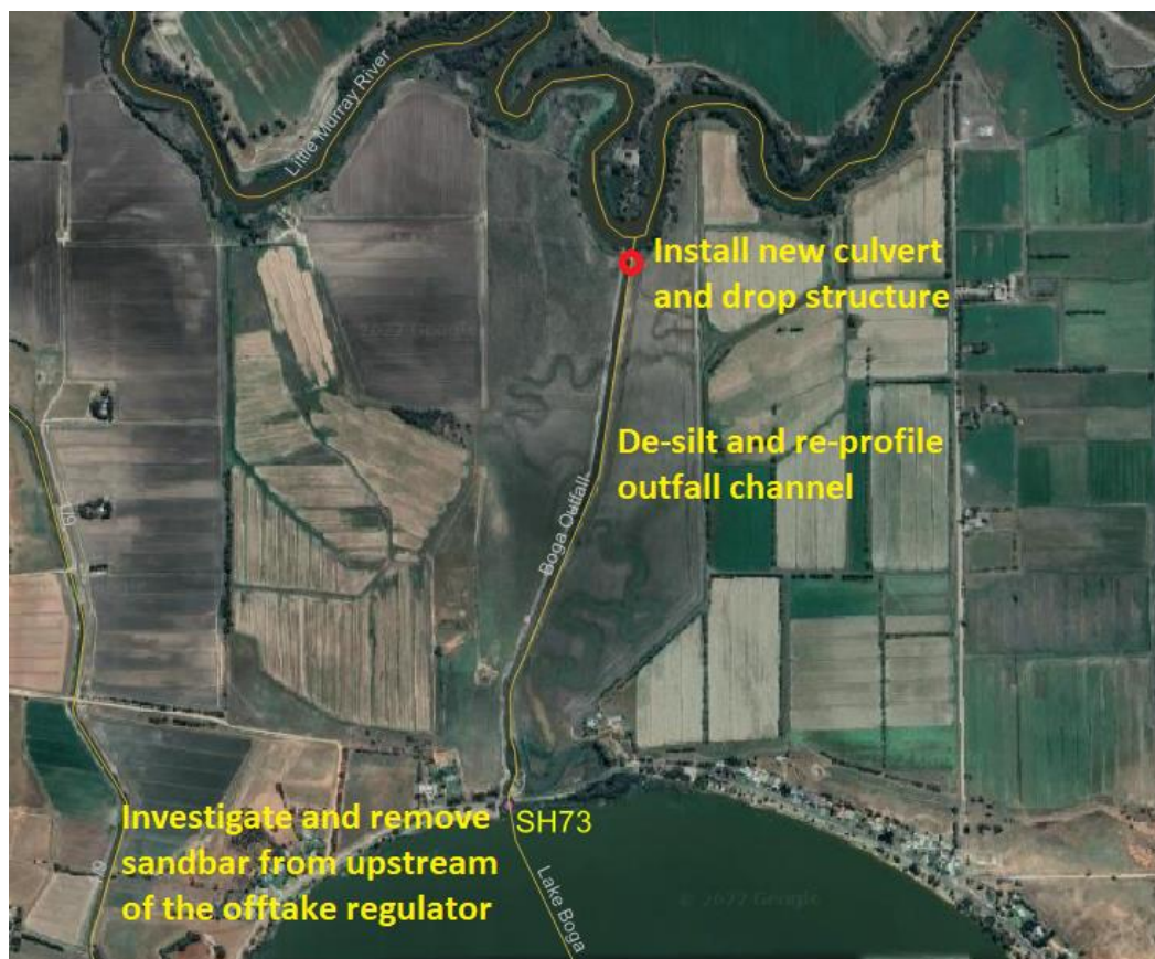
Figure 16. Proposed scope of works to reinstate the discharge capacity from Lake Boga
