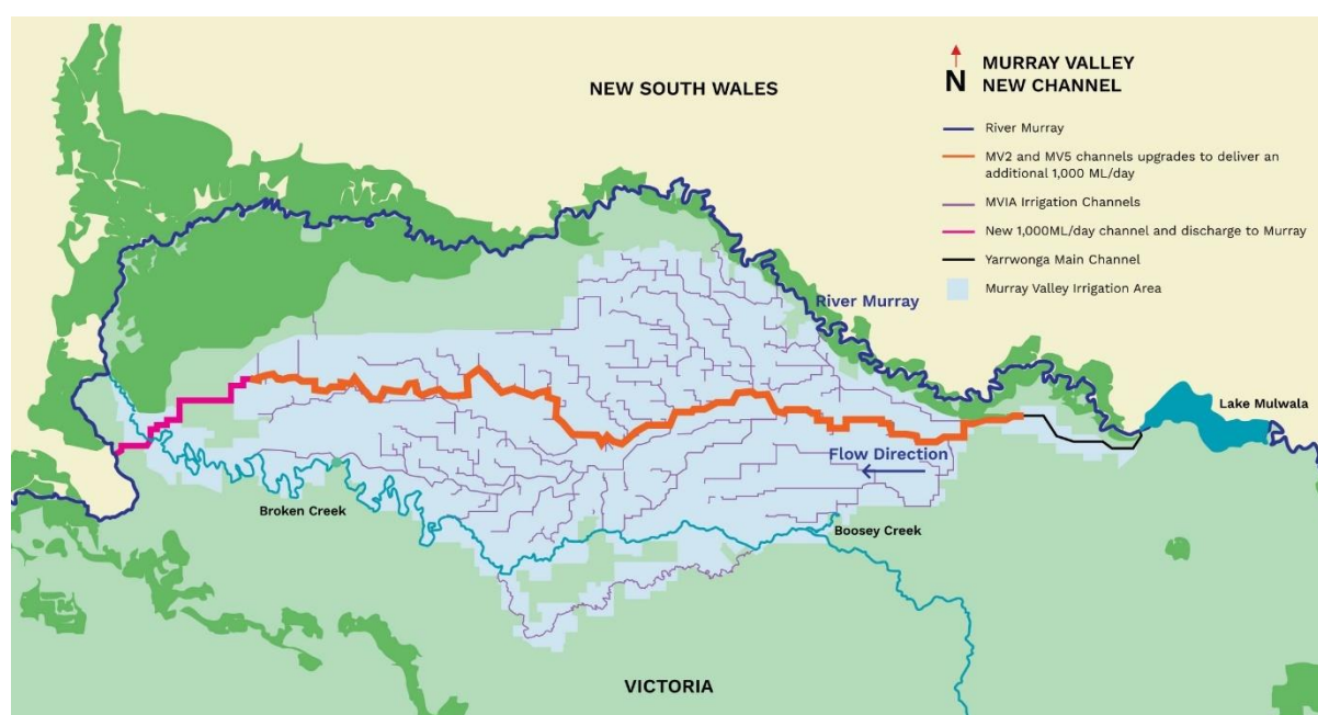
Figure 30. An indicative alignment for a channel to be constructed from Lake Mulwala to the River Murray
