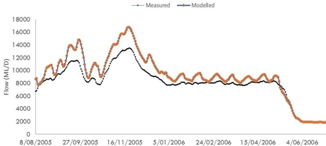
**Figure 23. Observed and simulated flows at Gauge 409215 below the Broken Creek confluence**
