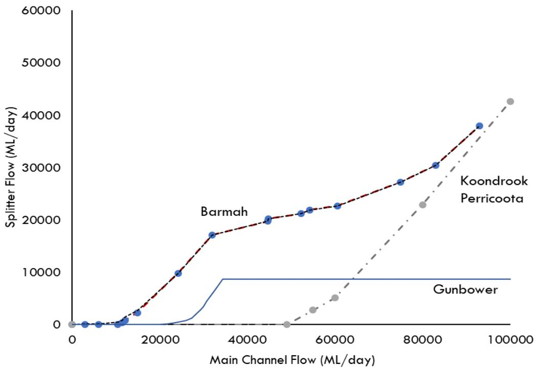
Figure 12. Splitter controlling flows to the Barmah and Gunbower floodplains
