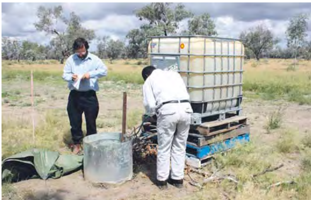
Boama Amofo (NSW Office of Water), right, and David Watson (Public Works NSW) undertaking infiltration testing at the disposal Basin site for the upper Darling salt interception scheme
