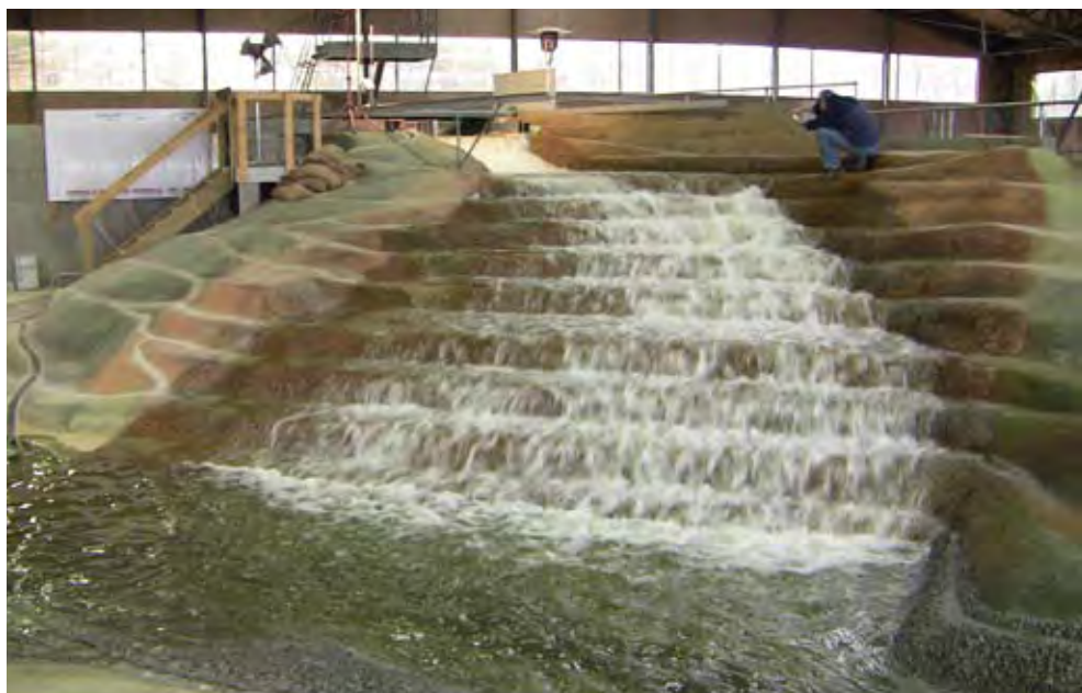
Hydraulic model of Dartmouth Dam in action. The model is being used to test the design of upgrades to the dam.
