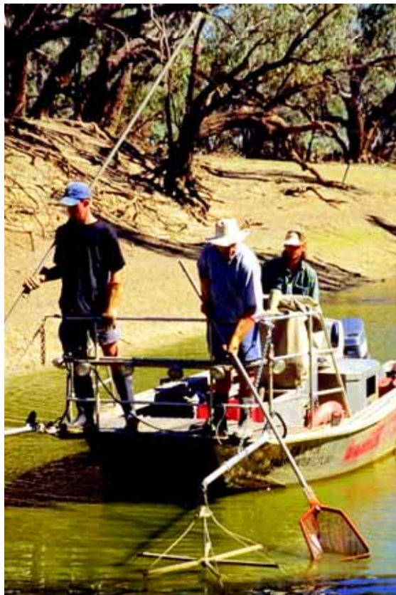
Boat electrofishing: Sampling for fish using boat electrofishing
