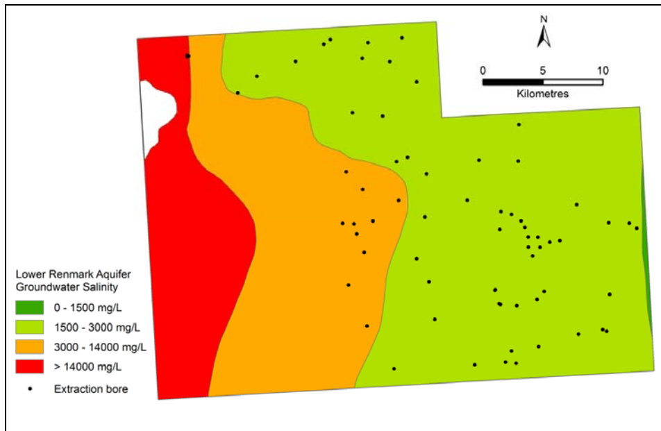
Figure 7. Peake-Roby-Sherlock Renmark Group aquifer salinity distribution, from the Lower Renmark salinity layer of the MDBA Basin in a Box dataset (MDBA, 2000)
