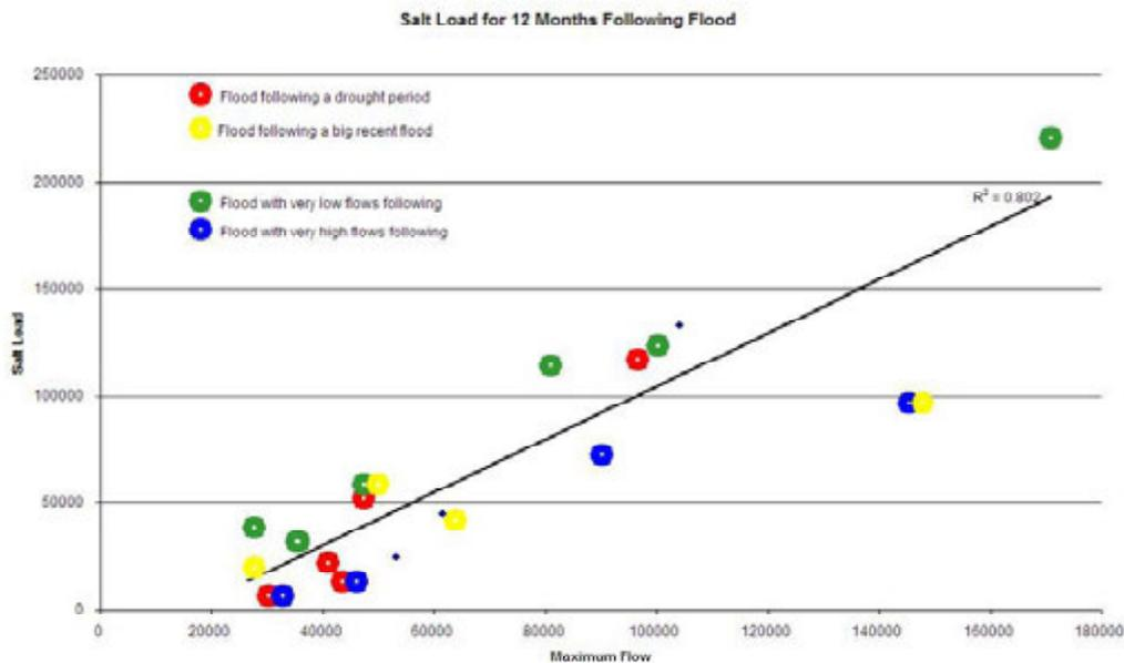
FIGURE 3.4: LINEAR RELATIONSHIP BETWEEN SALT LOAD (TONNES PER DAY) AND RIVER FLOW (ML/DAY) FOR CHOWILLA (FROM OVERTON *ET AL.* 2005)
