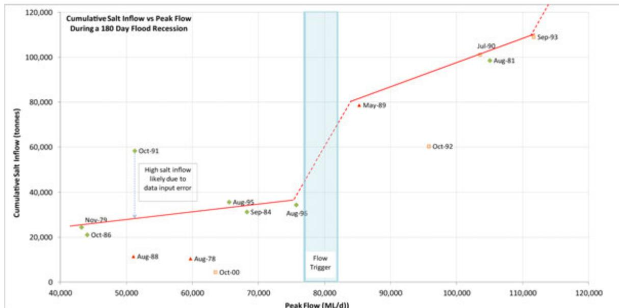
FIGURE ES.1: CUMULATIVE SALT INFLOW VS. PEAK FLOW DEMONSTRATING STEP WISE SALT INFLOW CONCEPTUAL MODEL
