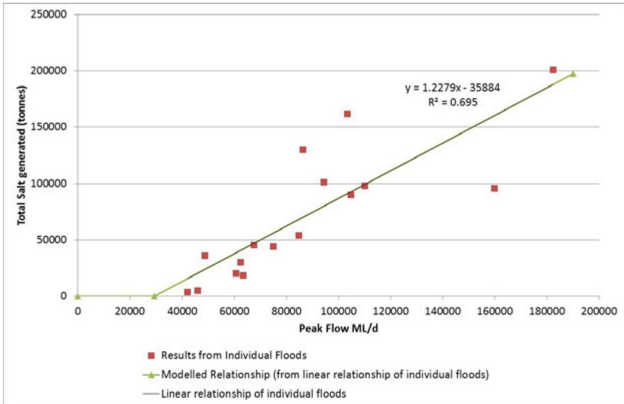
Figure 6: Relationship between peak flow and total salt generation. The parameter “salt generation factor” was set equal to the slope of the relationship. The parameter “salt event threshold” was set equal to the intercept of the relationship divided by the salt generation factor.
