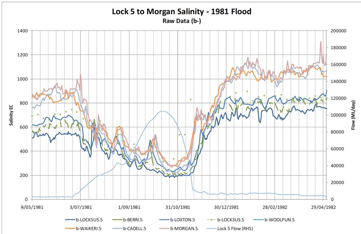
FIGURE 5.9: RAW SALINITY DATA FOR THE 1981 FLOOD
