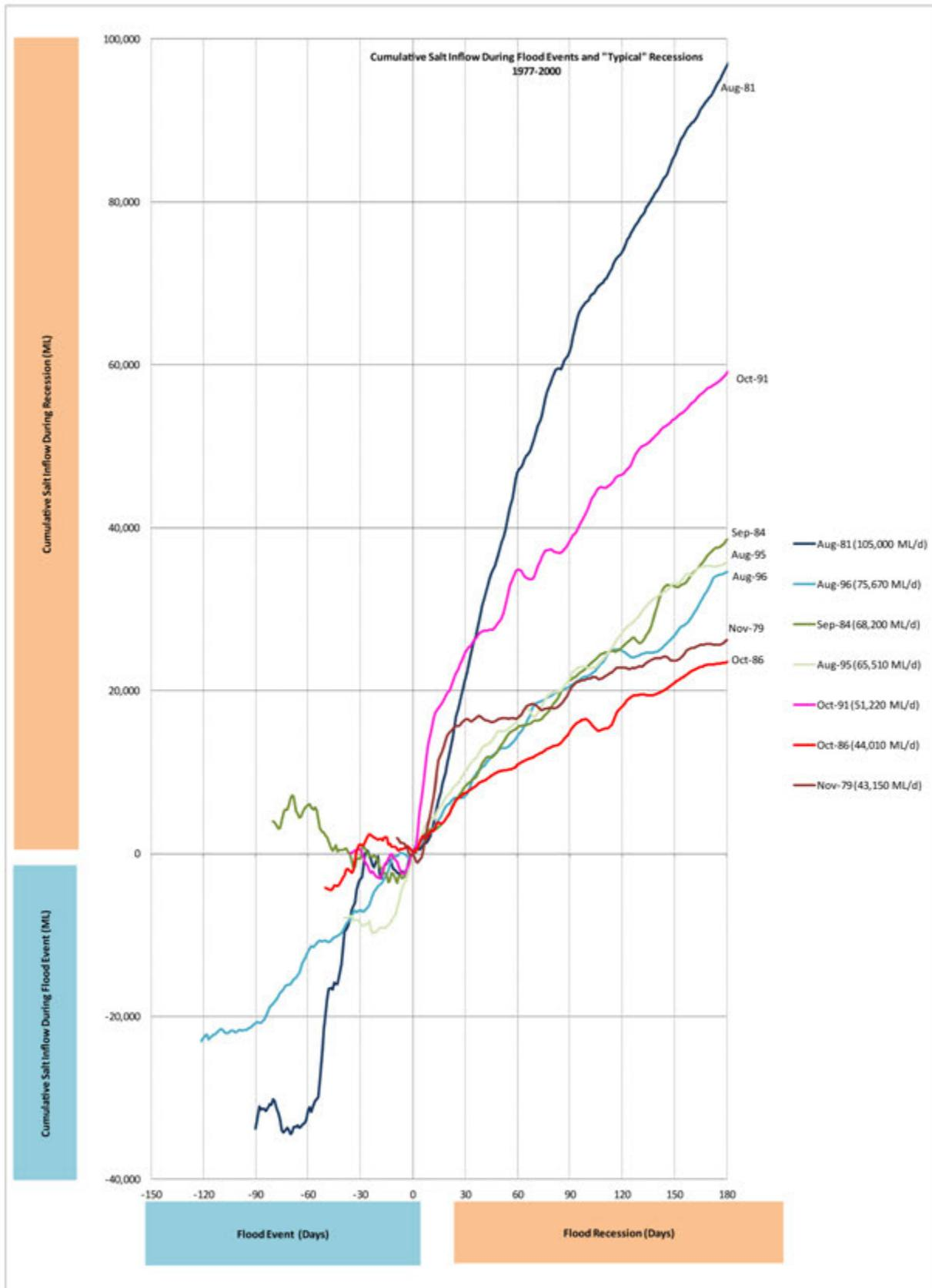
FIGURE 3.8: CUMULATIVE SALT LOAD DURING FLOOD AND "TYPICAL" RECESSIONS
