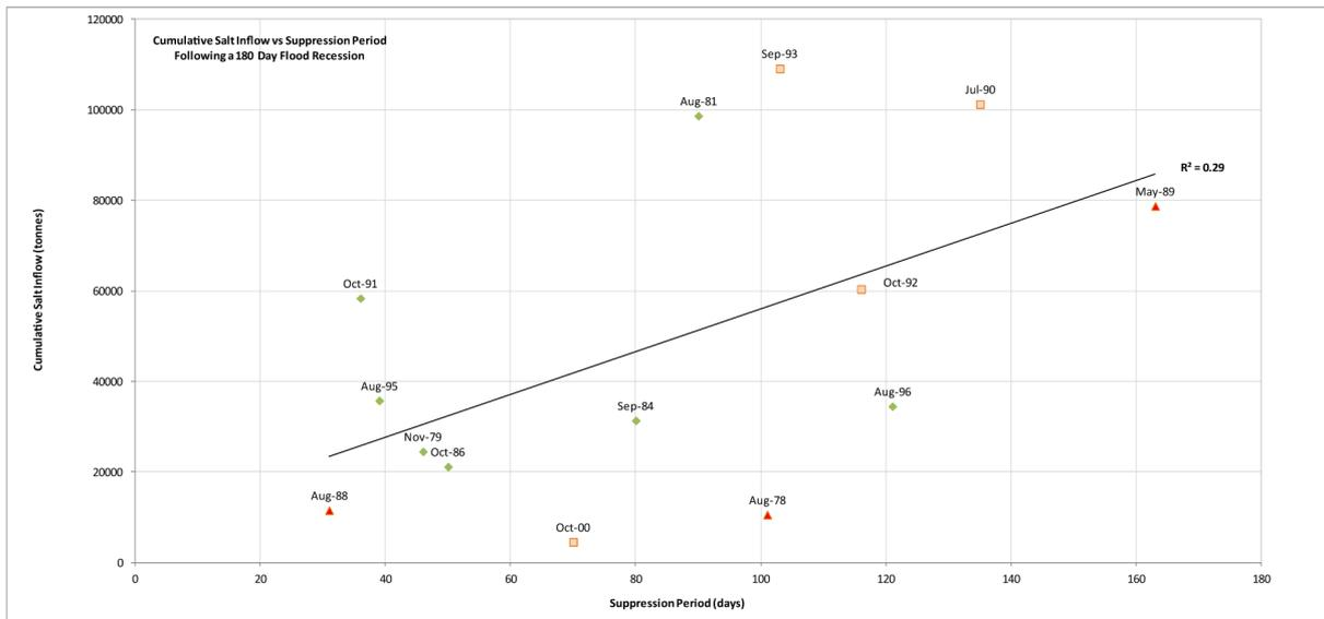
**FIGURE 3.17: RELATIONSHIP BETWEEN CUMULATIVE SALT INFLOW AND SUPPRESSION TIME FOLLOWING A 180 DAY FLOOD RECESSION**
