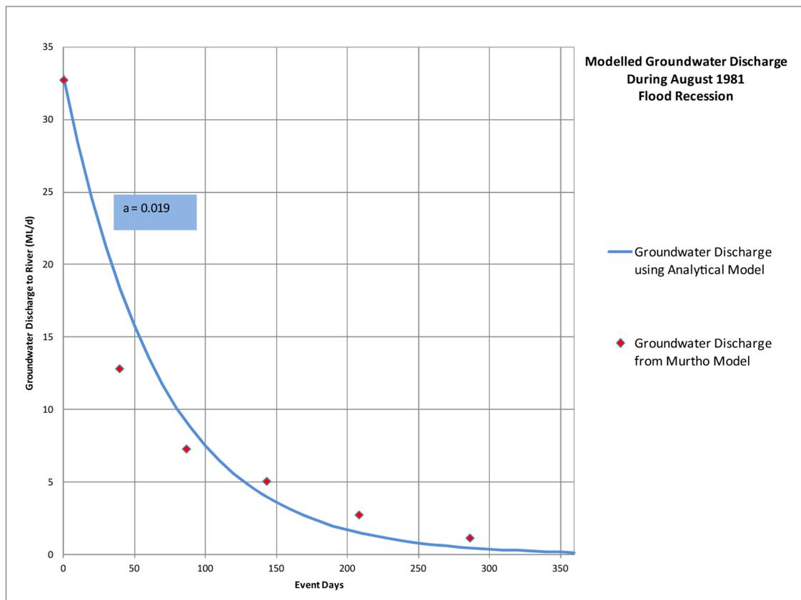
FIGURE 4.2: GROUNDWATER DISCHARGE TO RIVER DURING THE 1981 FLOOD RECESSION FROM MURTHO FLOOD MODEL
