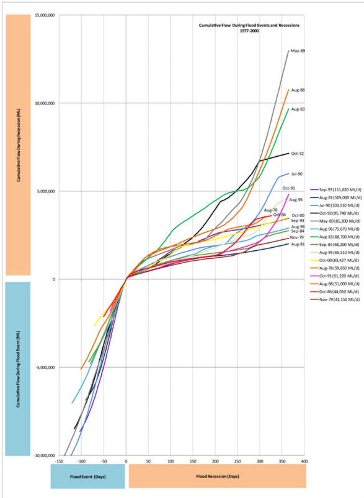
FIGURE 3.5: CUMULATIVE FLOW DURING FLOOD AND RECEPTION ORDERED BY FLOOD PEAK FLOW
