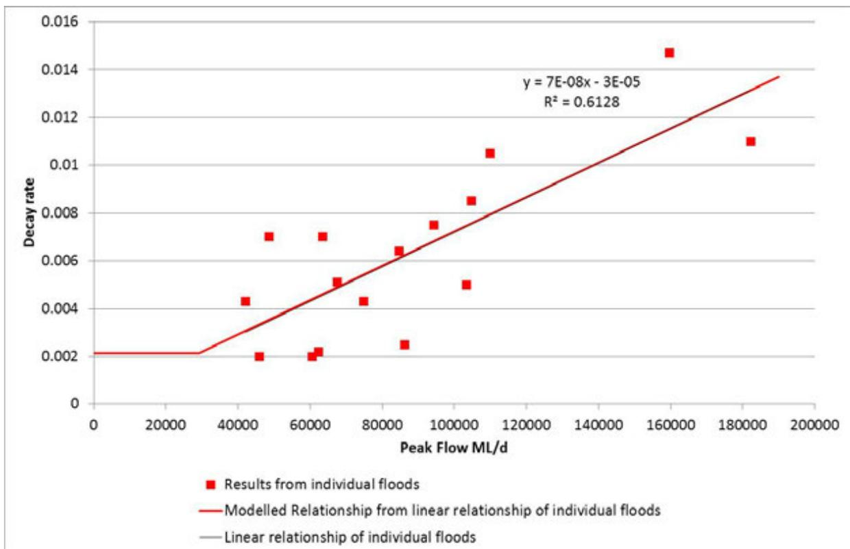
Figure 10: Relationship between peak flow and decay rate. The parameter “based decay rate” was set equal to the intercept of the relationship. The parameter “increase in decay rate with flow” was set equal to the slope of the relationship.
