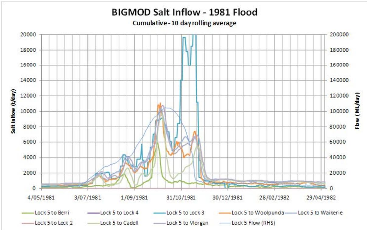
FIGURE 5.10: BIGMOD CALCULATED SALT INFLOW FOR THE 1981 FLOOD
