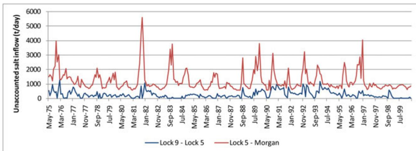
Figure 4: Time-series of unaccounted salt inflow for the region of focus for this Study: Lock 9 to Lock 5 and Lock 5 to Morgan.
