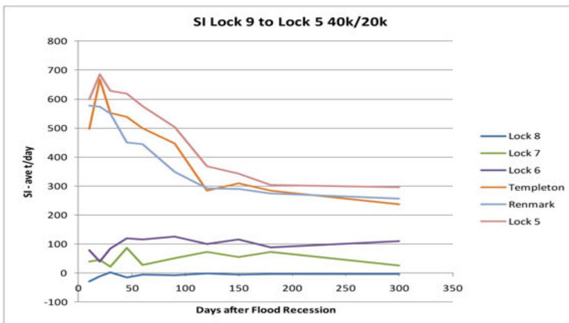
FIGURE 3.1: SALT INFLOW (LOCK 9 TO LOCK 5) VS TIME AFTER FLOOD RECESSON FLOWS FALL BELOW 20GL/D (AWE 2011)
