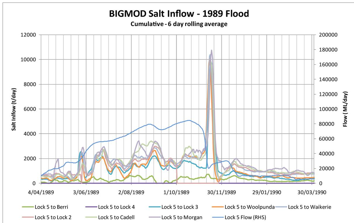
FIGURE 5.13: BIGMOD CALCULATED SALT INFLOW FOR THE 1989 FLOOD
