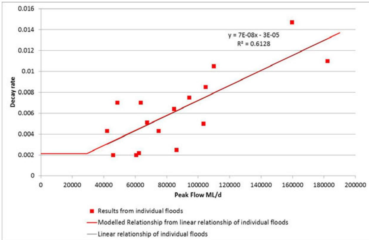
Figure 7: Relationship between peak flow and decay rate. The parameter “base decay rate” was set equal to the intercept of the relationship. The parameter “increase in decay rate with flow” was set equal to the slope of the relationship.
