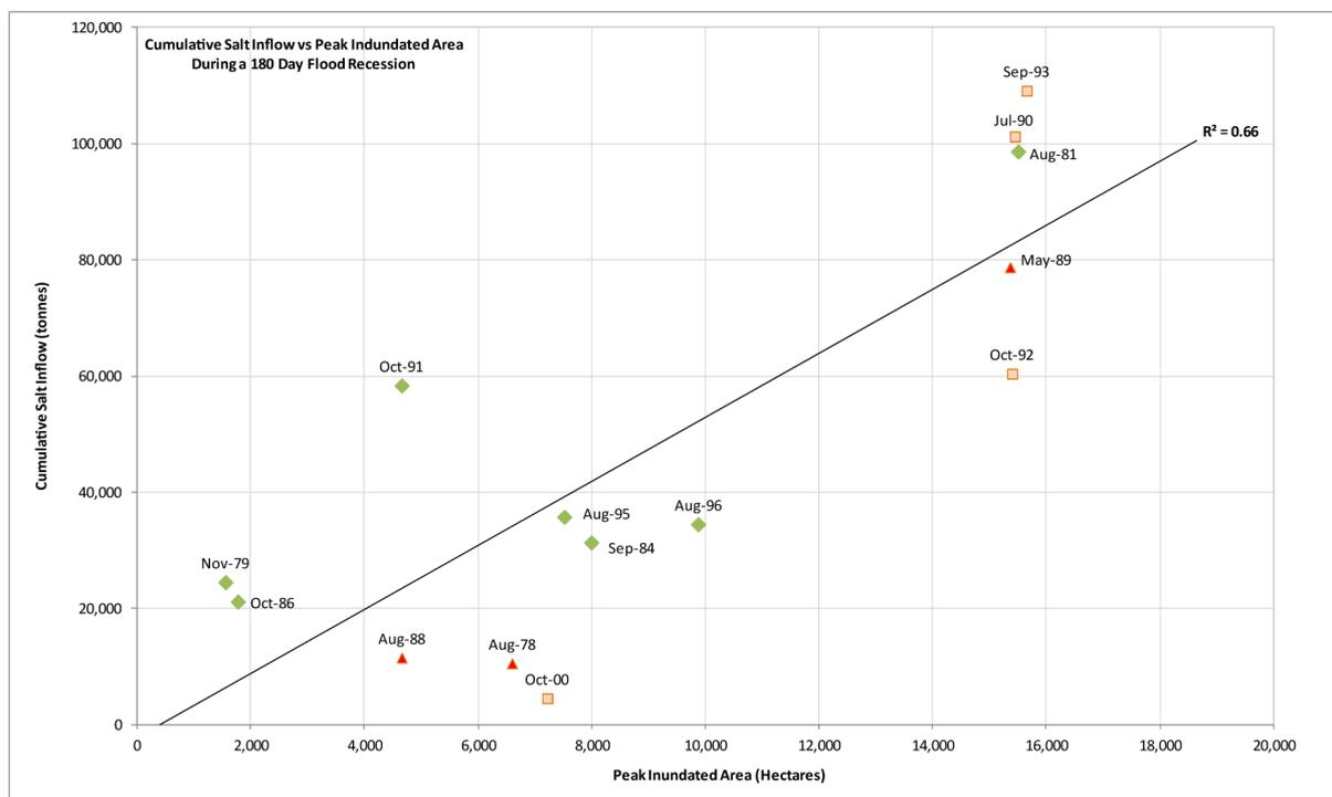
FIGURE 3.15: CUMULATIVE SALT INFLOW VS PEAK INUNDATED AREA FOR 180 DAY FLOOD RECESSION
