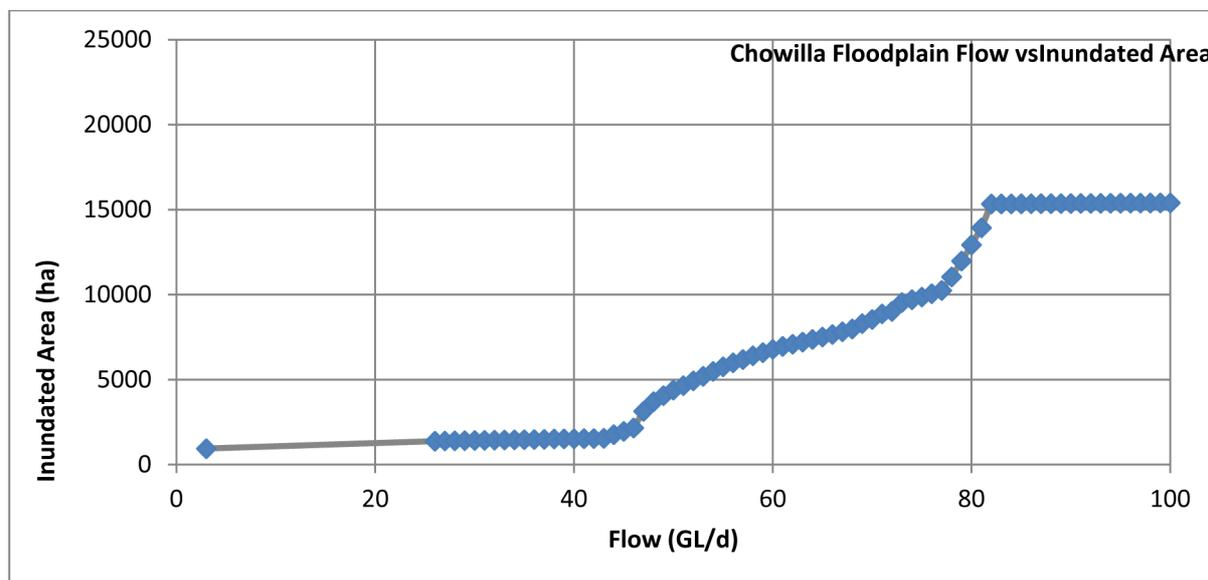
FIGURE 3.11: INUNDATED AREA VS FLOW FOR THE CHOWILLA FLOODPLAIN (AFTER RIMFIM MODEL)
