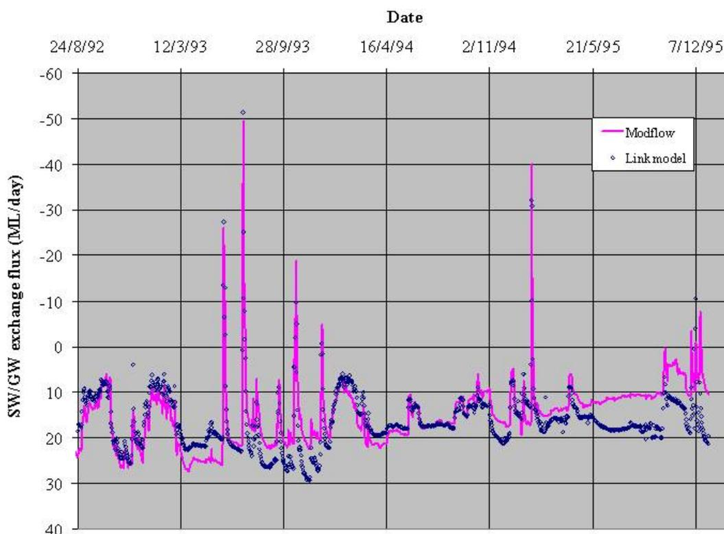
FIGURE 4.1: PRELIMINARY TRIAL RESULTS OF THE GROUNDWATER LINK MODEL AND CALIBRATED MODFLOW MODEL IN THE BOGGABRI TO NARRABRI REACH OF THE NAMOI RIVER (JOLLY ET AL. 2010)
