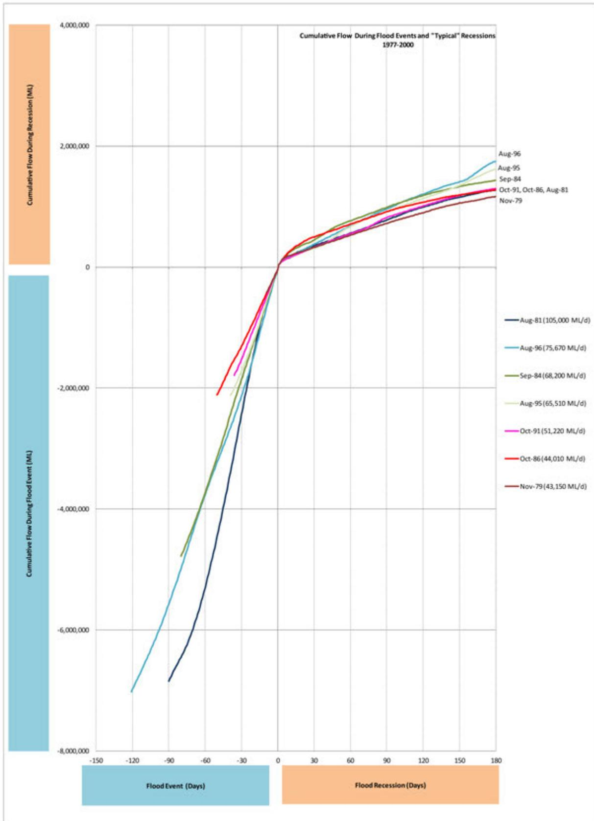
FIGURE 3.7: CUMULATIVE FLOW DURING FLOOD AND "TYPICAL" RECESSIONS
