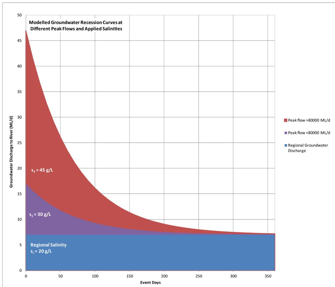
**FIGURE 4.3: MODELLED GROUNDWATER RESSION CURVES AT DIFFERENT PEAK FLOWS AND CORRESPONDING SALINITIES**
