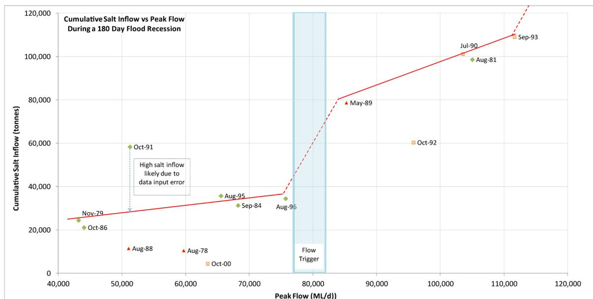
FIGURE 3.18: CUMULATIVE SALT INFLOW VS. PEAK FLOW DEMONSTRATING STEP WISE SALT INFLOW CONCEPTUAL MODEL
