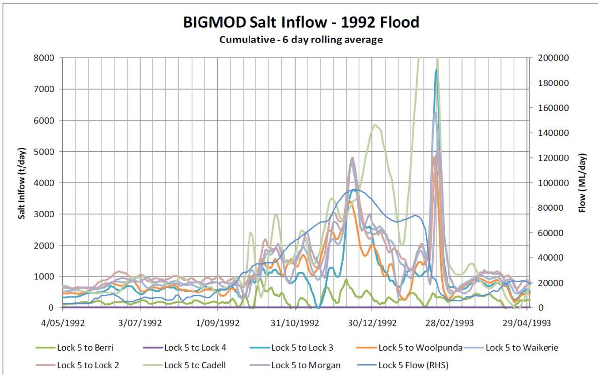
FIGURE 5.15: BIGMOD CALCULATED SALT INFLOW FROM THE 1992 FLOOD
