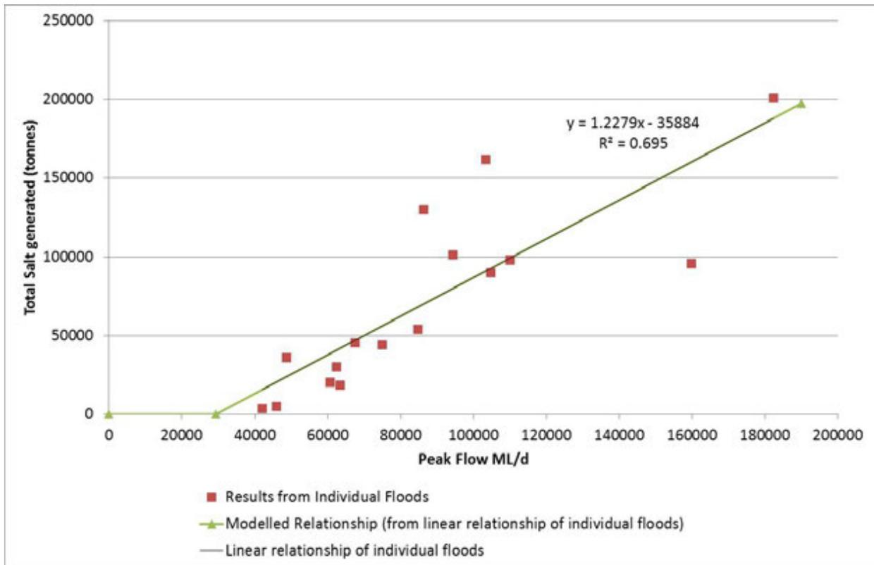
Figure 9: Relationship between peak flow and total salt generation. The parameter “salt generation factor” was set equal to the slope of the relationship. The parameter “salt event threshold” was set equal to the intercept of the relationship divided by the salt generation factor.
