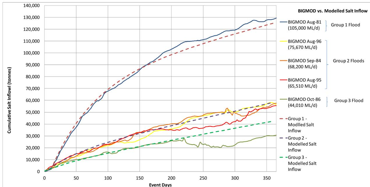
FIGURE 4.4: BIGMOD CUMULATIVE SALT INFLOW VS. MODELLED SALT INFLOW
