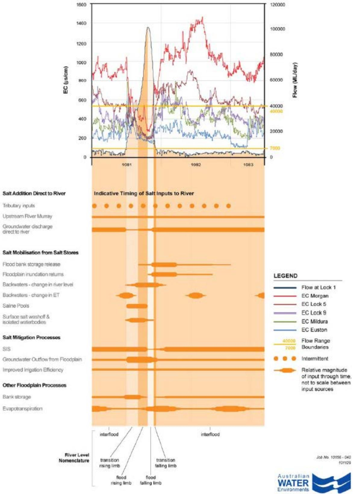
Figure 3: Indicative timing of salt inputs to the River Murray through a flood cycle (AWE 2012).
