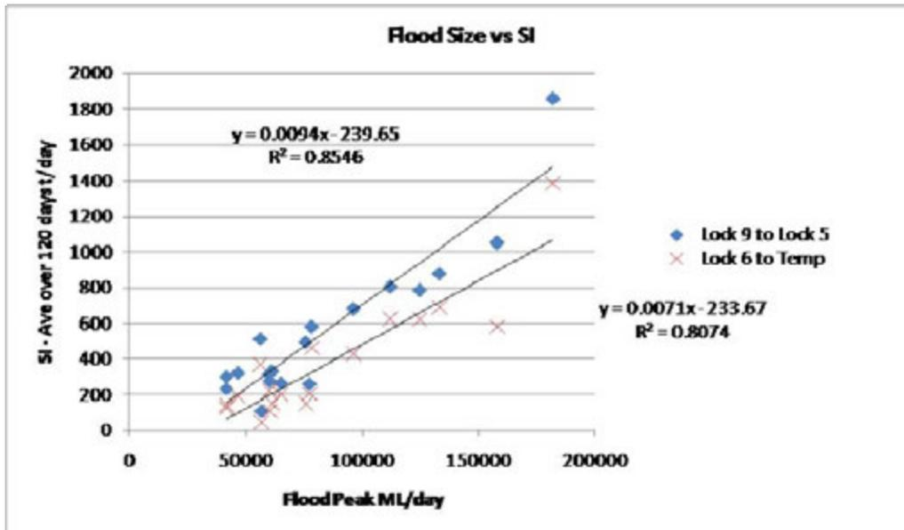
FIGURE 3.3: LINEAR RELATIONSHIP BETWEEN FLOOD PEAK FLOW AND SALT INFLOW (120 DAYS) (AWE 2011)
