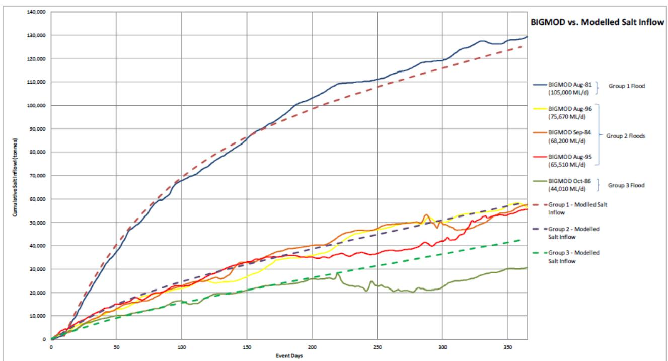
Figure 5: Comparison of BigMod cumulative salt input and modelled (simple analytical model) salt input (AWE 2013).
