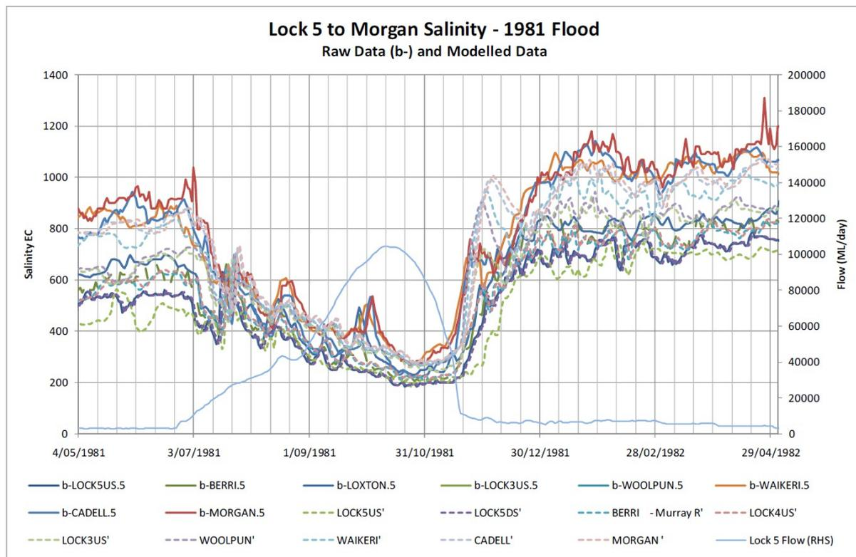
**FIGURE 5.11: RAW SALINITY AND BIGMOD CALCULATED SALINITY FOR THE 1981 FLOOD**
