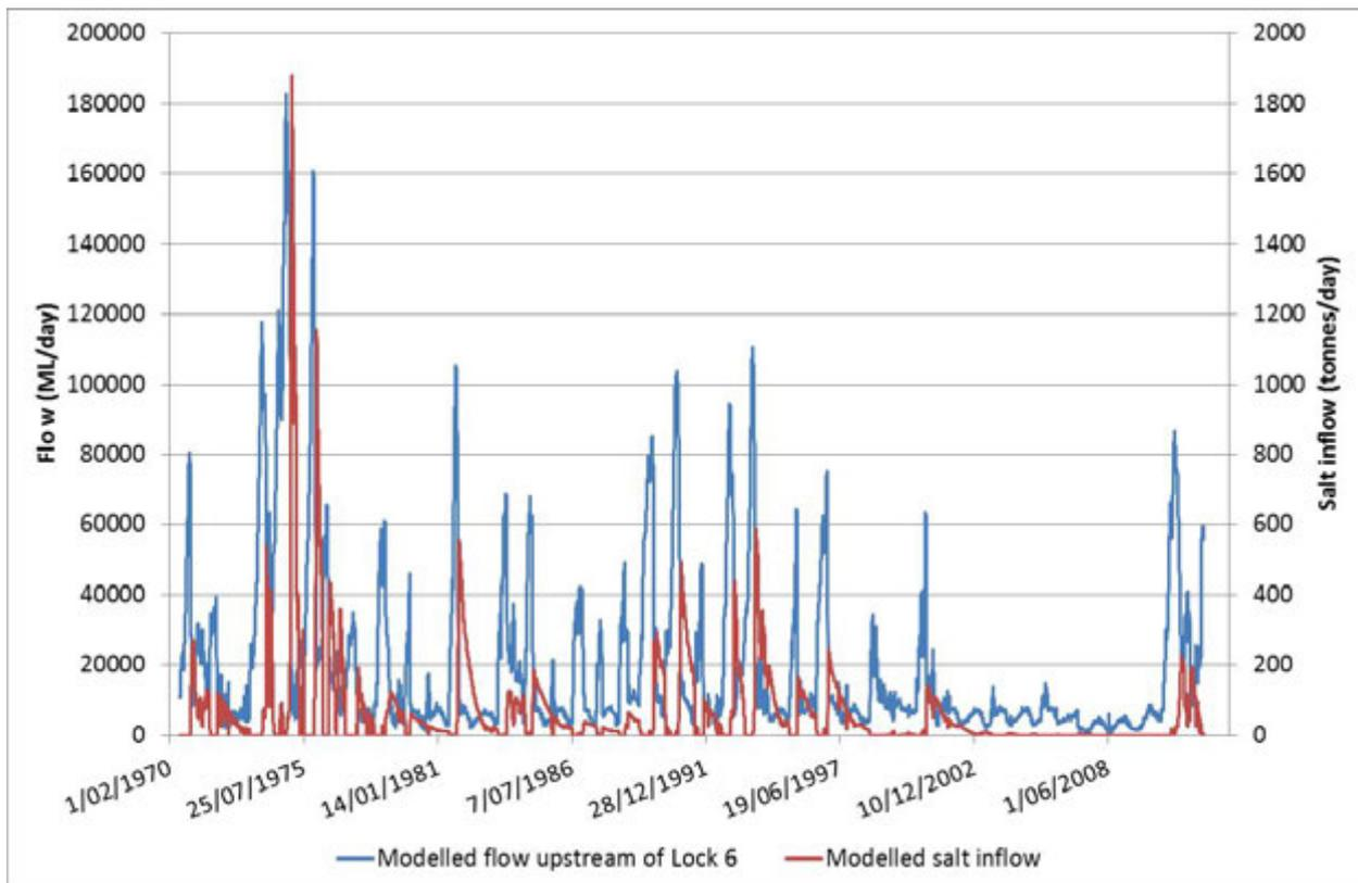
Figure 11: Time-series plot of modelled flow upstream of Lock 6 and salt inflow calculated by the proposed relationship.
