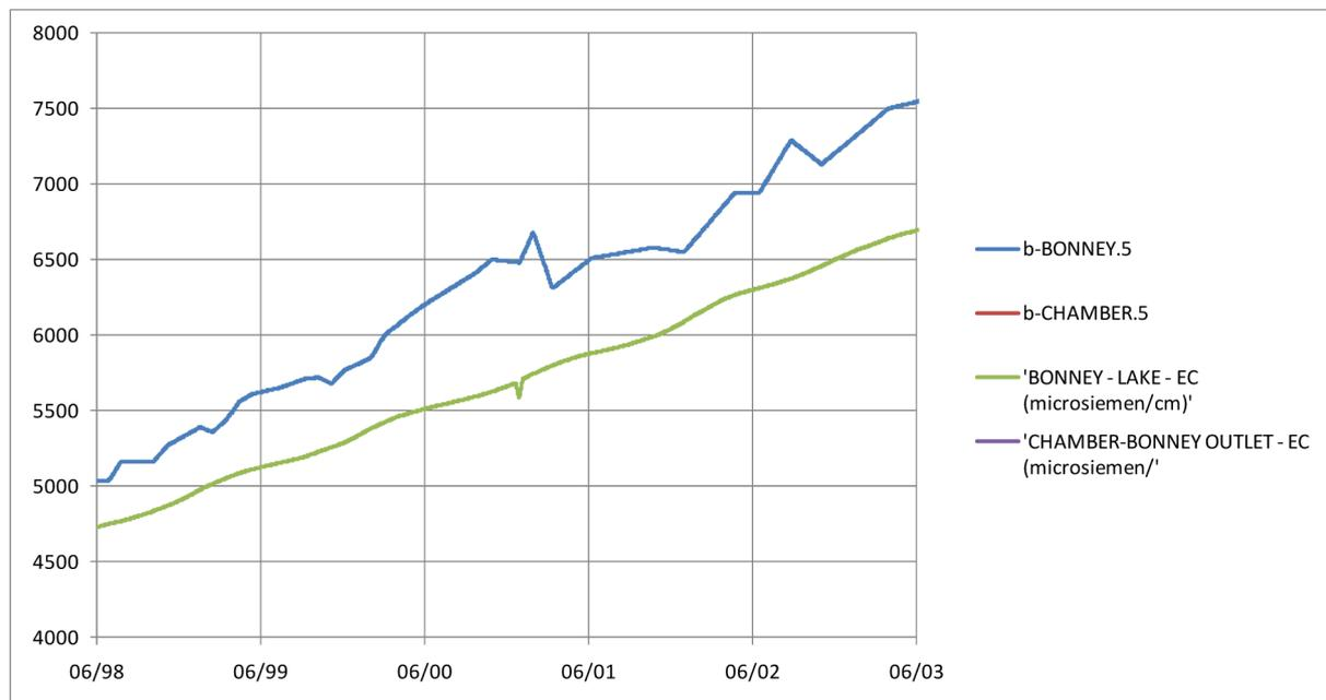
FIGURE 5.5: LAKE BONNEY SALT ACCUMULATION AND OUTFLOW TO THE RIVER 1998 TO 2003
